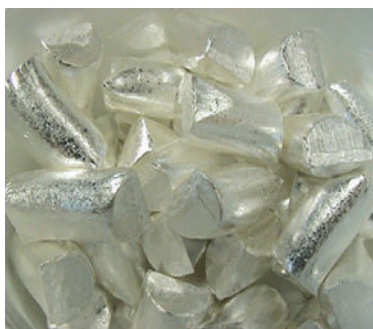
Ag 5N \varnothing 13.5 x 25 mm slugs
