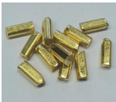
AuAs 0.4% \varnothing 5 x 11.1 mm slugs
