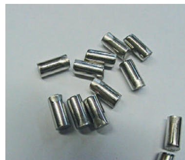
Pd \varnothing 2 x 4 mm slugs
